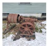
There were 8 wire cables connected to the frame of the elevator car that went up and over the Spoked wheel on the drive machine and then down to a counterweight to balance the load on the drive wheel. This elevator may have been driven by a water wheel in the river that most of the factories of the time used to power machinery, however looking at the
